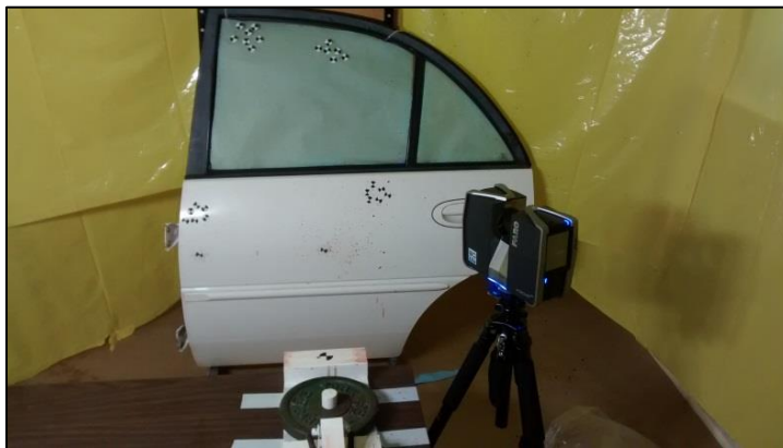
Figure 1. Car door with scanner and at the bottom of the picture is the bloodstain rig
