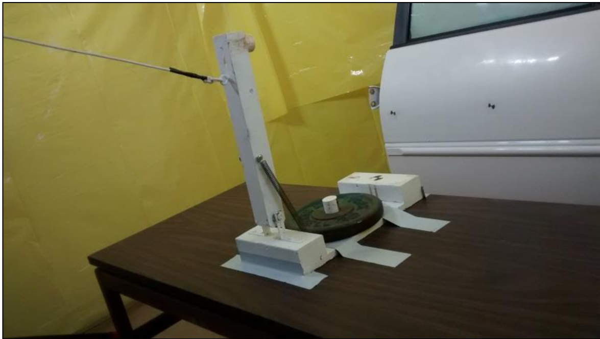
Figure 2. Bloodstain rig in an open position ready to create a bloodstain pattern
