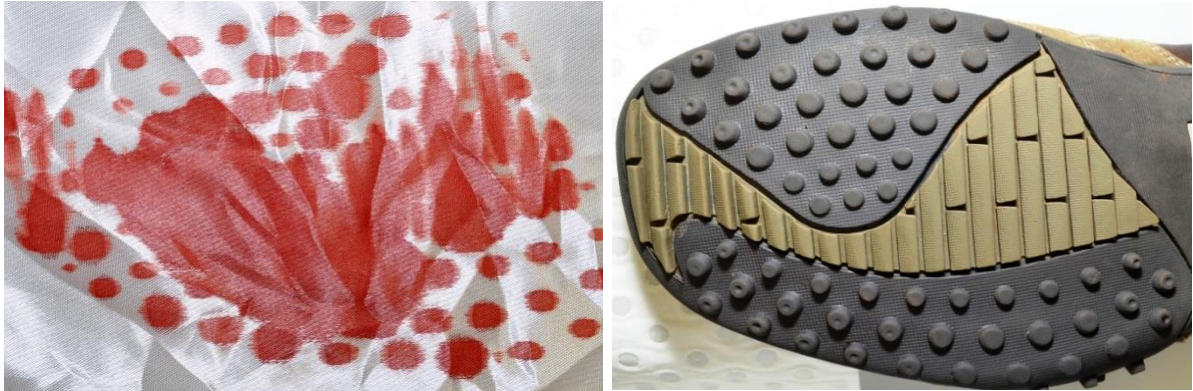
Figures 9 and 10. The transfer pattern (Figure 9) produced by the outsole (Figure 10) shows the shape of the stains is changing. The stains created by the raised round elements of the outsole are diffusing to form square shapes.
